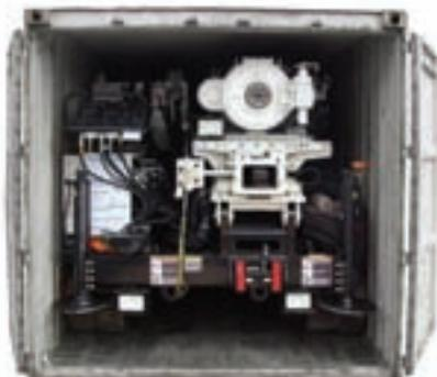
Meet the SDC-350 – a sonic drill rig that can fit within a 20' shipping container!
