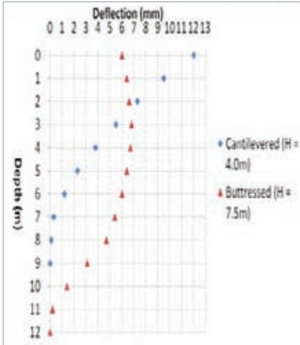
Site 2 comparison of deflections in the free standing cantilevered section with wall movement in the buttressed area
